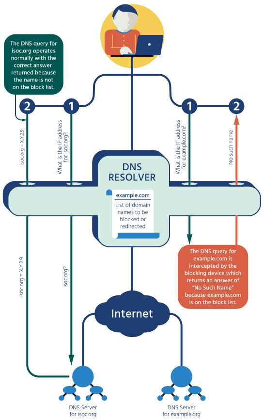
In DNS-based blocking, the blocking device has a list of DNS names to block.
